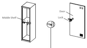
Connect the locker door to the small tab attached to the middle shelf. The door uses a spring loaded hinge pin.
