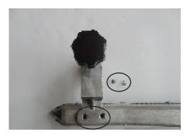
1. Remove the two tiny screws on each side of the main body and place the casters over the holes.
