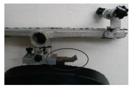
7. Slide the body of the nozzle onto the fixed bracket and secure with the star screw.
