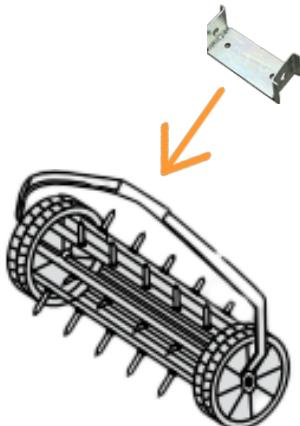
3. Next, place the steel adaptor on the top side of the aerator. Secure this in place with the nuts and bolts provided.
