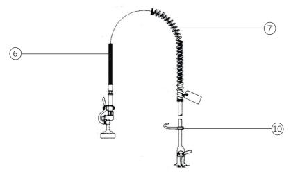
6) Adjust the position of no. 10 so that no. 1 hangs loosely in it without straining no. 6 or no. 7.
