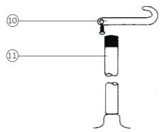
4) Screw no. 8 down onto no. 11. Tighten no. 8 with a wrench- this will consequently tighten no. 11.
