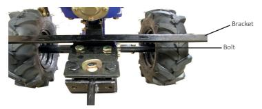
2. Attach the 2 short black attachment bars to the left and right hand side of the tiller, using a small bolt and nut.
