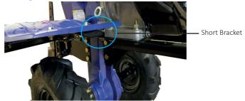
3. Attach the blue mud guards to the brackets. Use 4 x bolts and 4 x nuts per each guard.
