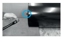
Place a metal arm onto the end of the roller's shaft.
