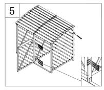
**Step Seven:** To attach the latch, mark the desired position onto the divider panel as shown in diagram 6. Line up the two parts of the latch onto the door on the line you have just made and screw into place using the provided 3\*16 screws.
