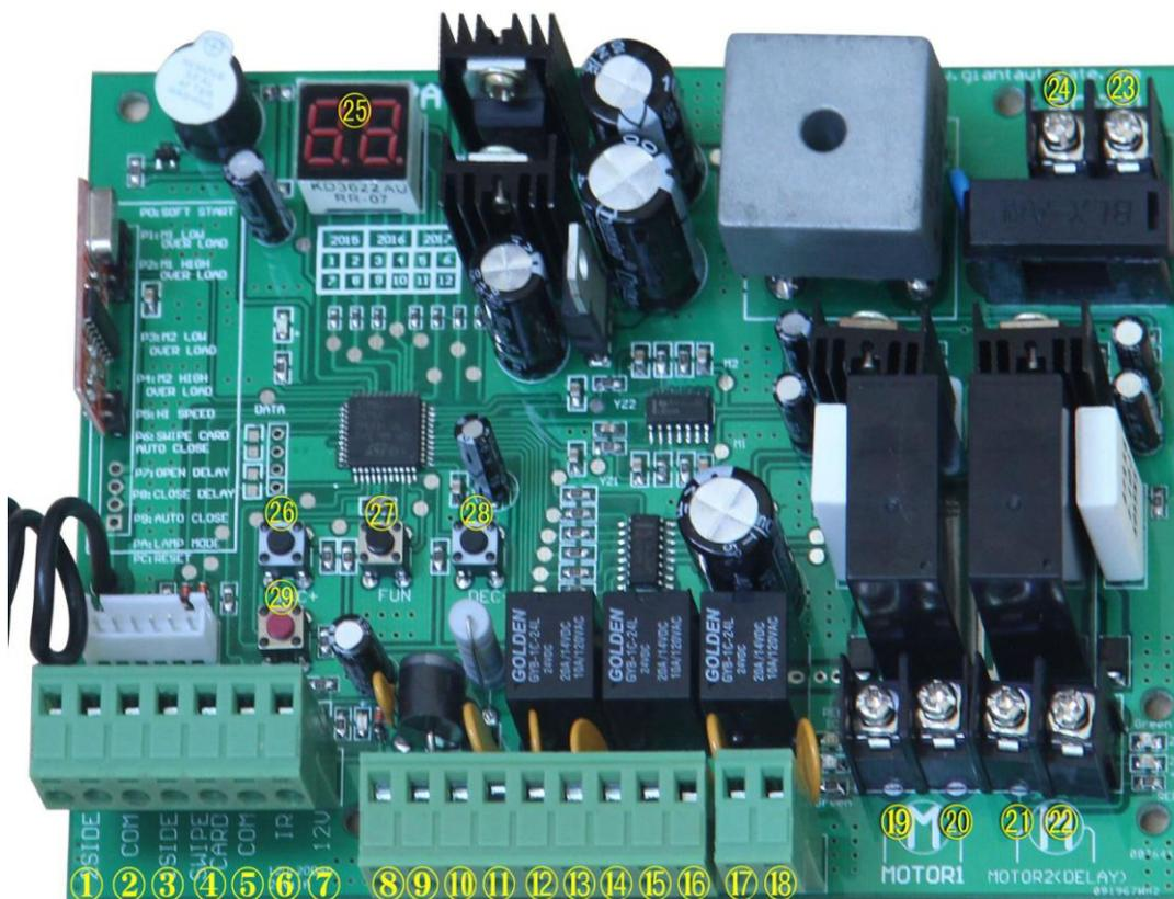
1. 2 SIDE terminal is used for connecting any external device that operates double gate
