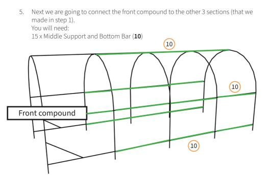
When attaching the Bottom Bars (**10**) and Support Bars (**10**) to the completed sections they need to be located on the inside of the polytunnel.
