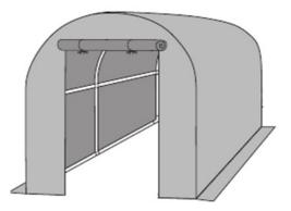
9. Finally, before attaching the Guy Ropes (**14**) we advise digging a trench to sink your poly tunnel into the ground.
