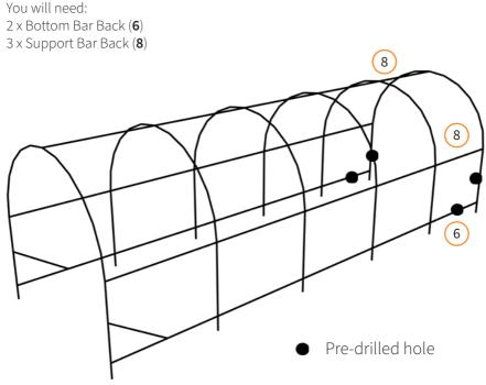
When attaching the Bottom Bars Back (6) and Support Bars Back (8) to the completed sections they need to be located on the inside of the polytunnel.
