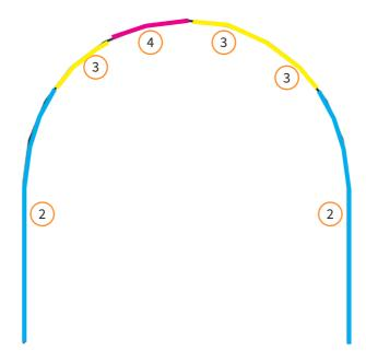
You will need to repeat this 6 times to make 6 complete sections like this. First and last section will be done according to the diagram above. For the middle sections, please use the **8 x Middle support Bars (5**) instead of the Uprights **(2**). 3. Next we are going to connect 2 of the completed sections together. For the purposes of these instructions this will be the front compound of the polytunnel. You will need:
