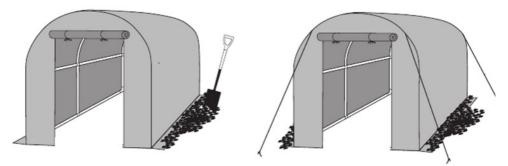
Once you have dug your trench, move the poly tunnel into place and cover the exposed cover at the bottom of the polytunnel with dirt.
