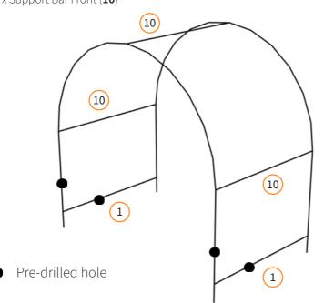
When attaching the Bottom Bars Front (1) and Support Bars Front (10) to the completed sections they need to be located on the inside of the polytunnel.
