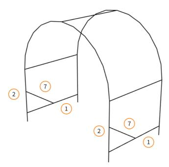
Attach one end of the Diagonal Support Bar (**7**) to the Upright (**2**) and then the other end into the predrilled hole on Bottom Bar Front (**1**). Repeat this step to attach both Diagonal Support Bars (**7**).
