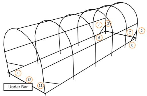
Attach one end of the Diagonal Support Bar (7) to the Upright (2) and then the other end into the predrilled hole on Bottom Bar Back (6).
