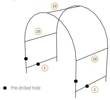
When attaching the Bottom Bars Front (1) and Support Bars Front (10) to the completed sections they need to be located on the inside of the polytunnel.
