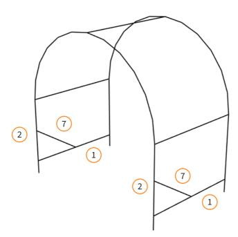
Attach one end of the Diagonal Support Bar (7) to the Upright (2) and then the other end into the predrilled hole on Bottom Bar Front (1).
