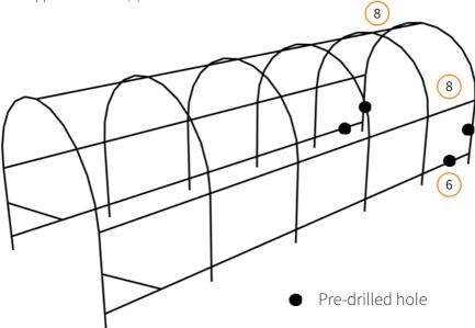
When attaching the Bottom Bars Back (6) and Support Bars Back (8) to the completed sections they need to be located on the inside of the polytunnel.
