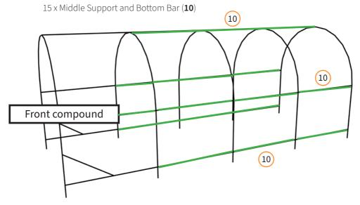
When attaching the Bottom Bars (10) and Support Bars (10) to the completed sections they need to be located on the inside of the polytunnel.
