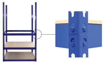
8) Then continue to build the rest of the shelves, attaching the short beams at the side first, then the long beams at the front and back. Slot in each of the remaining MDF boards as you go.
