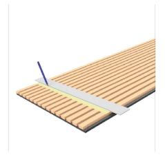
Measure and mark location of cut on the panel. Apply a strip of masking tape along area to be cut. Strike a line across using a pencil and straight edge.
