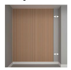
Repeat the above procedure for all remaining full width panels. When you come to the end of the run, it may be necessary to cut the last panel to the correct width. Measure the distance from the edge of the panel to the wall, at top and bottom, to check it's parallel.
