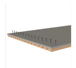
If slats on panel are loose after cutting, secure slats by inserting 15mm long screws through back of panel, through the felt and into the slats ensuring that screw heads are flush with back face of felt backing. Check panel fit on wall.
