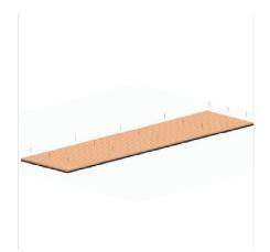
To secure the panel to the wall using screws, you will require 15 off, 3.5mm x 35mm black drywall screws set in 5 rows of 3. Top and bottom screws should be placed no closer than 50mm from the ends. On a 2.4m panel, rows should be spaced approx. 575mm apart. Using black coloured screws will help the screw heads blend in with the black backing felt.
