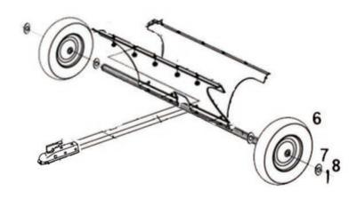
4.Mount the wheels(Part 7) and washer on both sides, Insert the pin.
