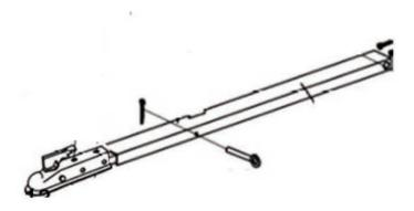
7.Insert pin into tow bar and fixed by a "B" shape pin
