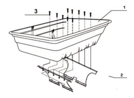
1.Connect the potect plate(part 2) and the tray(part 1) with screws and nuts(part 3).
