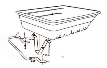
6.Connect the leg(part 9) whole handle and the tray with screws and nuts.
