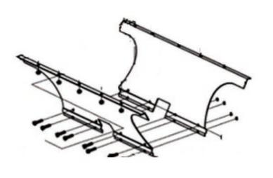
2.Connect 2 protect plates with screws and nuts.
