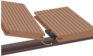
3. Start laying your decking boards at the outside of the area to be decked. Place your first board and screw it into each joist it crosses using a row of starter clips. Then fit T-Clips into the groove along the side of the board and screw them into each supporting joists with the screws provided, one T-Clip for each supporting joist.
