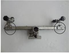
2. Replace the screws. Two on each side. The casters should sit as pictured.
