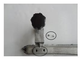
1. Remove the two tiny screws on each side of the main body and place the casters over the holes.
