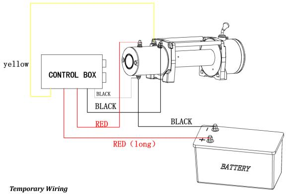
1. Lift the rubber seal, and plug the POWER CABLE into the PLUG on the right side of the winch body. This plug is labeled "power". Route the Power Cable from the winch to your battery, being
