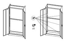
5) The frame should now look like the picture below (shown without doors). Notice that the apex of the cross on the Rear Panel (C) is towards the lower end of the frame.
