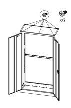
7) Notice that at the base of the frame, there are two catches at either side, where the Floor Panel (F) will sit. See the picture below. Lay the frame on its back and place the Floor Panel (F) into the frame. Fit into place. Underneath the base is the final screw hole. Align and use 1 x Screw (H). Ensure the base is even before screwing.
