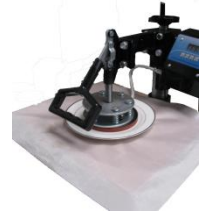
Figure 50: Lock the press down on the plate
