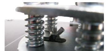
Figure 8: Press attachment with wing nuts
