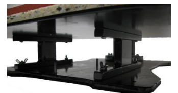
Figure 10: Base plate attachment with wing nuts
