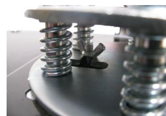
Figure 42: Press plate attached with wing nuts
