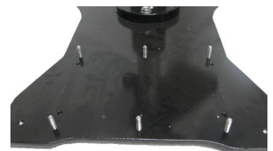
Figure 32: Main stand base with bolts for attaching the cap base stand
