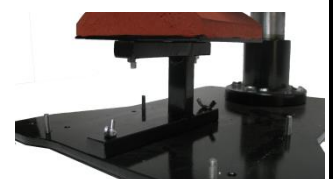
Figure 33: Cap base stand on middle two bolts
