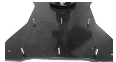
Figure 9: Main stand attachment plate with bolts for attaching the base plate
