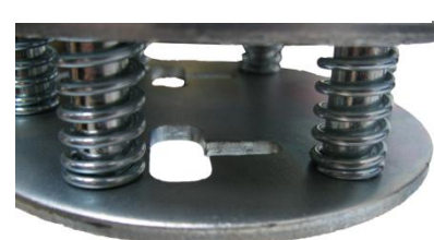
Figure 41: Central attachment- T shaped gap
