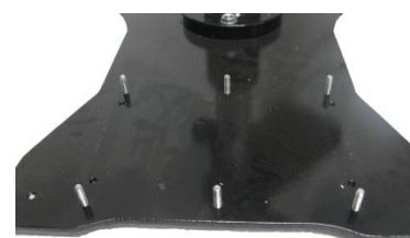
Figure 43: Metal base with bolts for base plate stand
