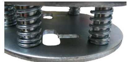
Figure 30: Central attachment- T shaped holes
