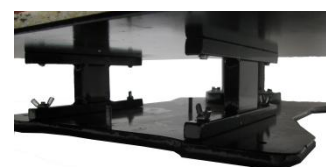
Figure 43: Metal base with bolts for base plate stand
