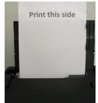
Figure 10: Sublimation paper correct printing side
