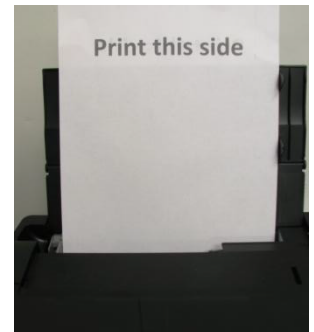
Figure 10: Sublimation paper correct printing side
