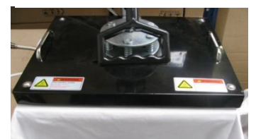
Figure 6: Heat press locked down on product
