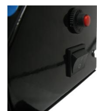
Figure 9: On/ off switch
