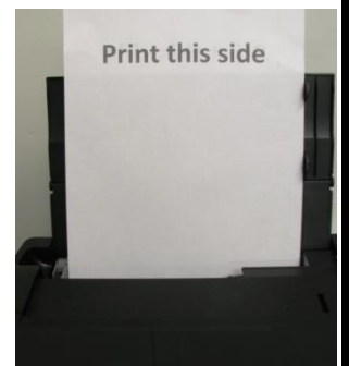
Figure 4: Sublimation paper correct printing side
