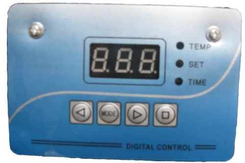
Figure 1: The control unit interface
