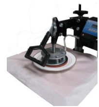
Figure 11: Lock the press down on the plate
