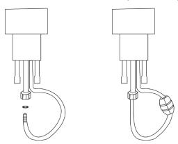
6) The tap is now ready to be installed. The nut ends of the hot and cold connectors can be attached to the isolator valves in your sinks assembly.
