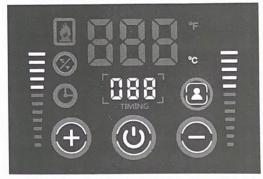
If not begin to countdown automatically when press the handle down, can press "-" button, to countdown manually. When the count down is over, the time shows "000". When hear the warning sound, means the transfer finish, then open the handle, take the mug out. Short press the "Start" button, hear "beeps" sound, turn off the machine.
