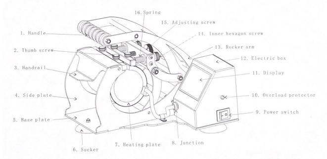
1. Start: Press the "Start" icon for two seconds, hear "beeps" sound, enter heating interface, start heating automatically. The default temperature is 190°C, and time is 180 seconds. When temperature reach to 190°C, will hear continuous warning sound, means the pre-heating temperature reached. Press the handle down, the sounds stop, will begin to countdown. During countdown process, press "+" to restart countdown. If not begin to countdown automatically when
