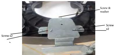
6. Secure the fixed bracket with four screws and one screw and washer as shown.
